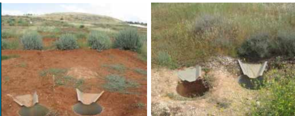
Figure 48. Measurement of runoff from exposed and treated areas at the ICARDA compound in Aleppo, Syria
