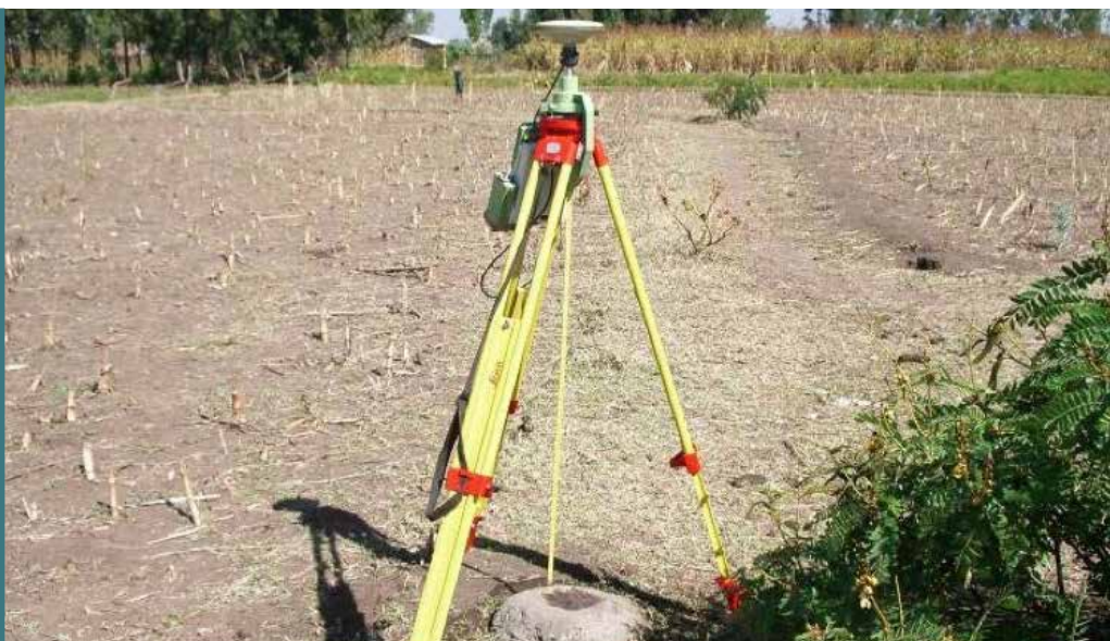
Figure 57. A parcel survey instrument - Precision GPS-RTK
